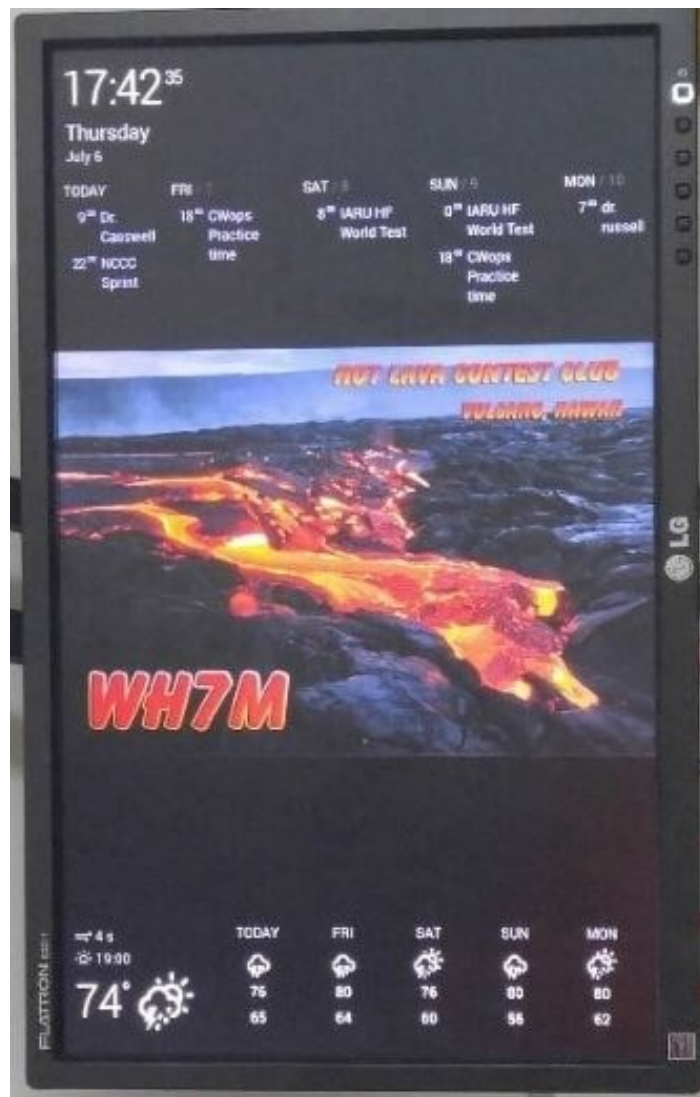
QSL card images are pulled from the cloud and overlaid with local weather, time, and calendar events
