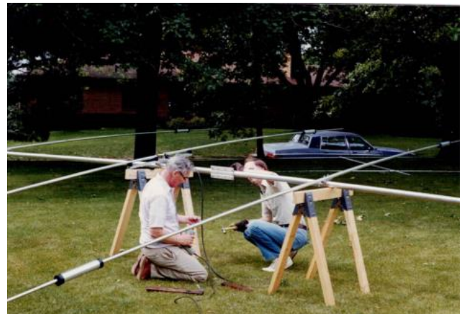
Early 2000s: W0TRF and W1GL assembling new Mosley TA-34
