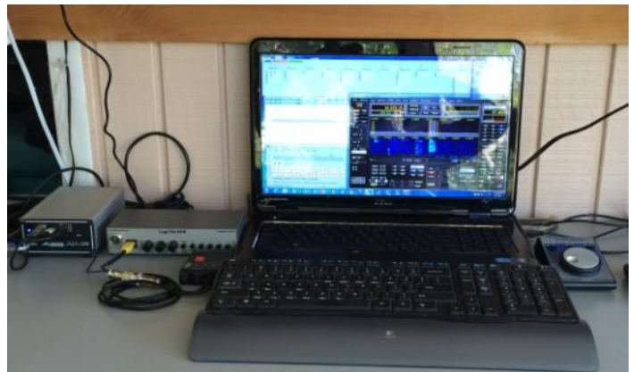
The simple, compact setup used by WØGJ at VP5H consisted of a Flex 1500, a LogiTalker Voice Keyer, an Azden PTT-02 VOX, and a laptop
