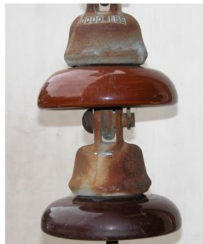
Arcing occurred between two of the three components in this insulator. It was a significant source of noise until it was replaced by utility personnel.
