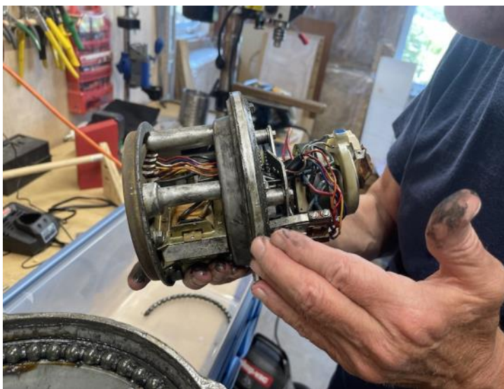
We disassembled the Ham IV rotor to see if there was a problem in it. There wasn't.
