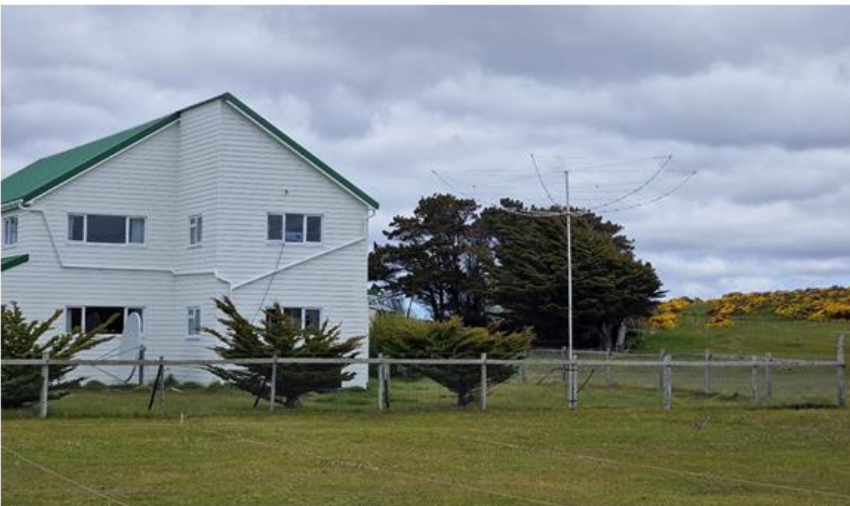
Figure 9 - Hexbeam on an approx. 5m tall mast which was fixed with straps to a pole of the fence.
